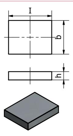
$\begin{array}{ll} b & = 6 \\ h & = 2 \\ I & = 7.5 \\ \text{Nominal adhesive forces} = 5 \\ \text{Weight in g} & = 1 \end{array}$
